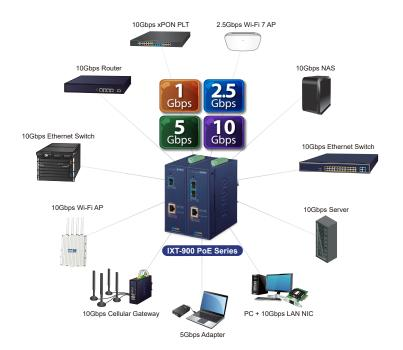
The fiber-optic **10GBASE-X SFP+** interfaces support 4 speeds, 10GBASE-SR/LR, 2500BASE-X, 1000BASE-SX/LX and 100BASE-FX, meaning the administrator now can flexibly choose the suitable SFP/SFP+ transceiver according to the transmission distance or the transmission speed required to extend the network efficiently.
